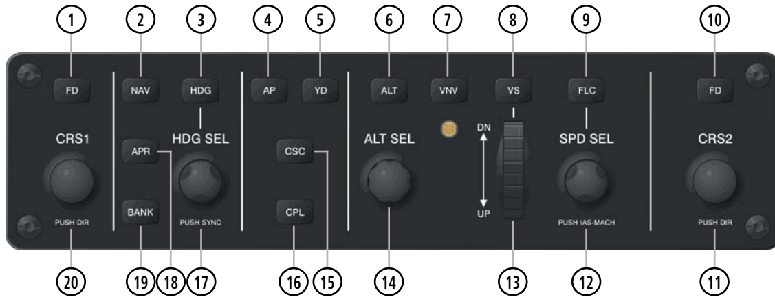
Figure 7-1 GMC 715 AFCS Control Unit
